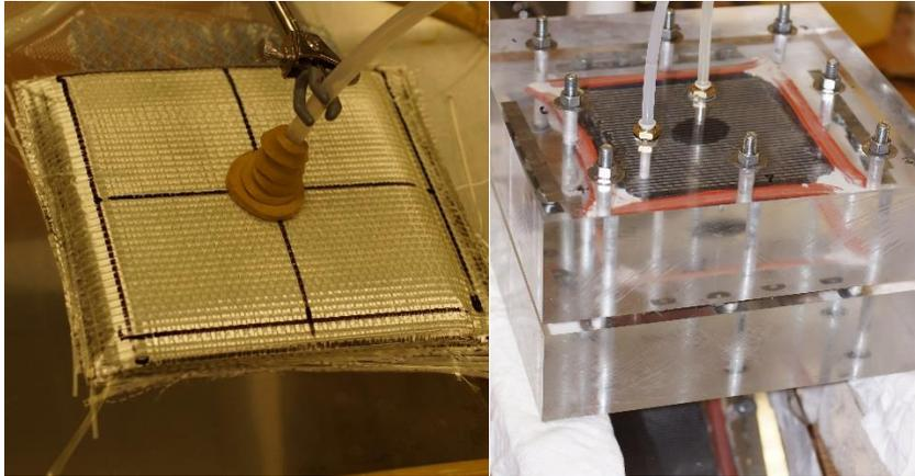
Figure 1: Permeability measurement tools: vacuum bag (left) and rigid (right).
